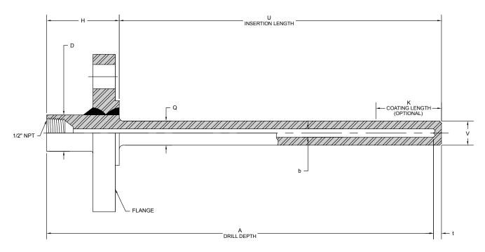
Daily Thermetrics' Model 130 Flanged Thermowells consist of a thermowell shank made from a single piece of solid bar stock welded to a flange. Raised face and ring type joint flange connections are available, and gaskets must be used during installation. Designed for use with thermocouples, RTDs, bimetallic thermometers, and other instrumentation devices (see Daily Thermetrics' Sensor Catalog). All aspects of the thermowell are customizable.
