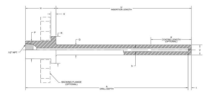
Daily Thermetrics' Model 140 Van Stone Thermowells are constructed from a single piece of solid bar stock and are designed to be in direct contact with the process. Raised face and ring type joint flange connections are available and gaskets must be used during installation. Designed for use with thermocouples, RTDs, bimetallic thermometers, and other instrumentation devices (see Daily Thermetrics' Sensor Catalog). All aspects of the thermowell are customizable.
