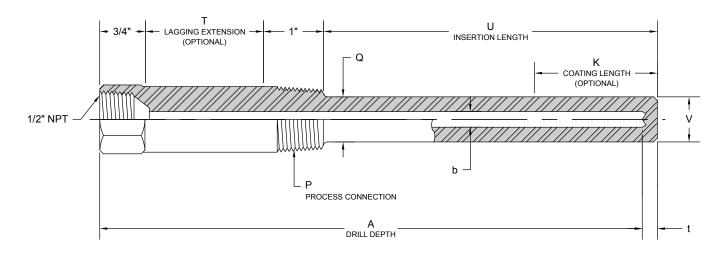
Daily Thermetrics' Model 110 Threaded Thermowells are manufactured from a single piece of solid bar stock and can be utilized with thermocouples, RTDs, bimetallic thermometers, and other instrumentation devices (see Daily Thermetrics' Sensor Catalog). All aspects of the thermowell are customizable.
